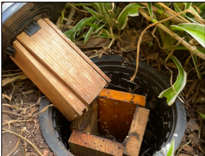
The TermiSensor is a device placed on top of termite monitors to detect termite activity and send notifications to the pest manager
