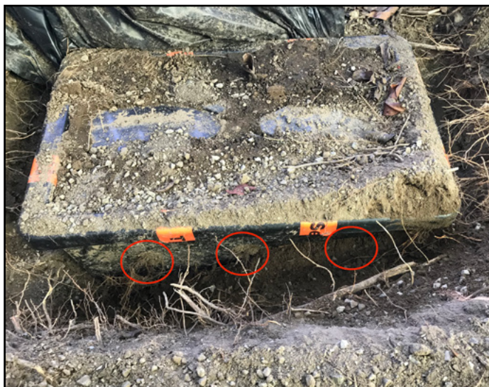
Plastic tubs containing foam samples, with holes in the side to allow termite access, were buried in the ground in Townsville in areas of high Mastotermes activity
